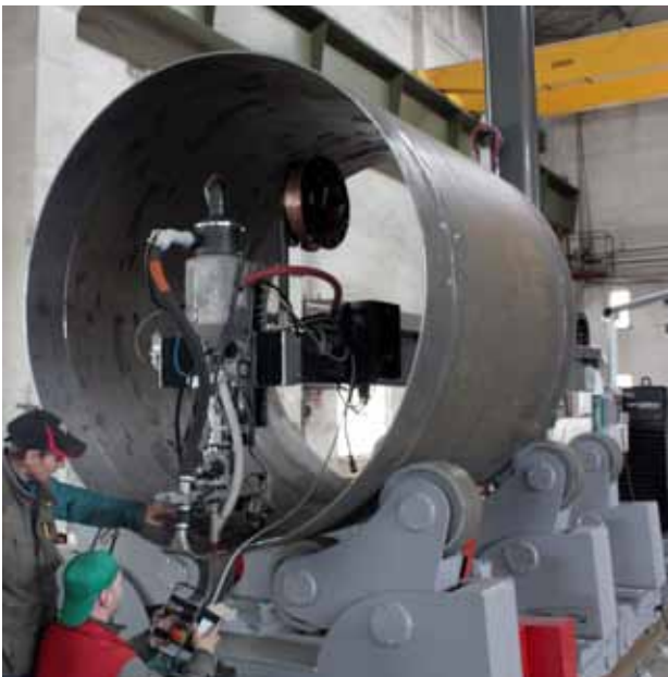
Internal longitudinal welding with PEMA column & boom and a set of roller beds
