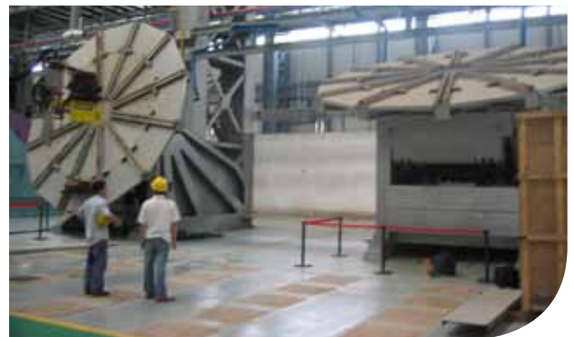
PEMA positioners commissioned at a customer site
